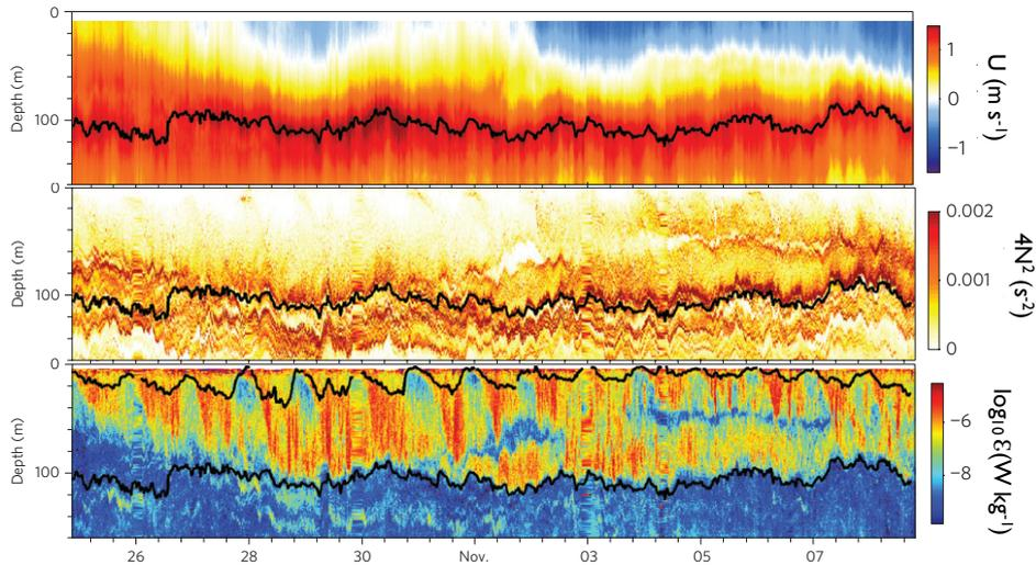
Figure 2: The rich structure of near-surface turbulence. Profiling time series at  $0^\circ, 140^\circ$  W in boreal autumn 2008, reproduced from *Moum et al.* (2009). (top) Zonal velocity: the core (eastward velocity maximum) of the eastward-flowing EUC is shown as a black line; (middle)  $4N^2$ ; (lower) turbulence dissipation rate,  $\epsilon$ . The mixed layer is defined by the upper black line in e as the depth at which  $\rho$  deviates by  $0.01 \text{ kg m}^{-3}$  from its surface value.
