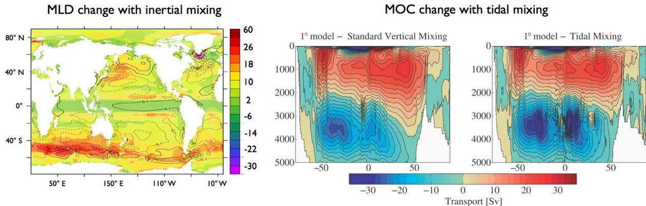
Figure 8: Examples of the sensitivity of large-scale circulation patterns to diapycnal mixing parameterizations in the upper and deep ocean. Left: change in mixed-layer depths, in meters, when near-inertial motions are explicitly represented in a global model, reproduced from *Jochum et al.* (2013). Right: snapshots of the modeled MOC using a standard parameterization for diapycnal diffusivity and one that includes elevated mixing over rough topography, reproduced from *Jayne* (2009).
