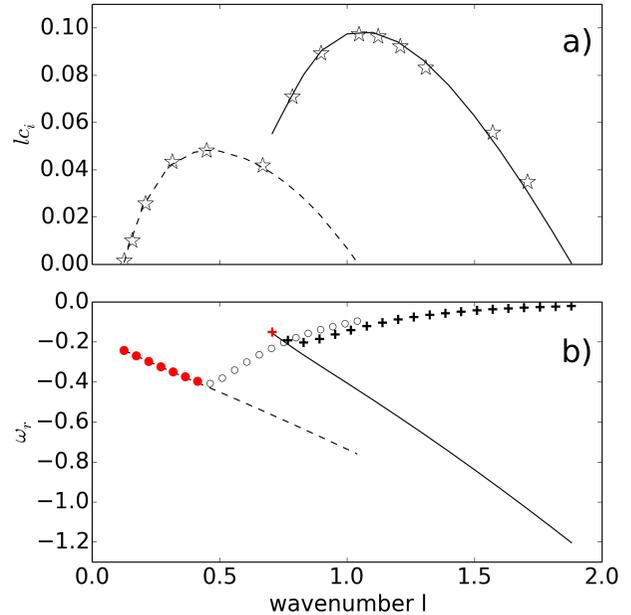
**Figure 1.1** (a) shows the growth rates calculated by a shooting method (lines) and an initial value method (stars). (b) shows the real frequencies calculated from eigenvalues,  $\omega_r = lc_r$  (lines) and  $\omega_r = -\beta^* k_r/(k_r^2 + l^2)$  where  $\beta^* = 0.41$  (symbols). In (a) (b), the dashed lines represent modified varicose modes, and the solid lines represent modified sinuous modes. The red symbols in (b) marks the unstable modes that satisfy the matching condition.
