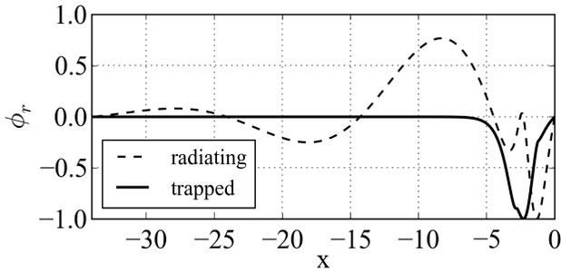
**Figure 1.2** The real part of the eigenfunctions of the radiating (dashed) and trapped (solid) modes as a function of  $x$  ( $x$  is normalized by  $L_b$ ). The radiating mode has  $l = 0.4$ ,  $k = 0.21 - i0.0011$ , and the trapped mode has  $l = 0.82$ ,  $k = 0.32 - i0.74$ .
