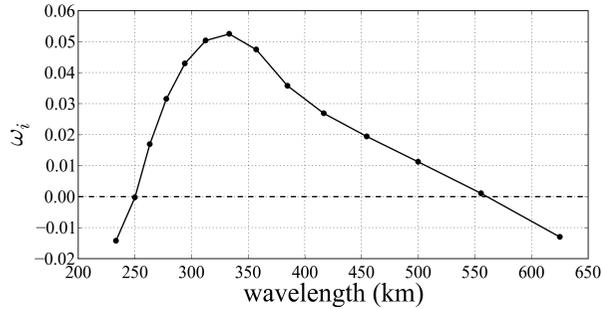
**Figure 1.3** Linear growth rates normalized by  $V/L_b$  as a function of meridional wavelength. The growth rates are calculated by fitting the time series of the integrated perturbation kinetic energy to exponential curves,  $EKE = Ce^{2\omega_i t}$ , where  $\omega_i = lc_i$  is growth rate.
