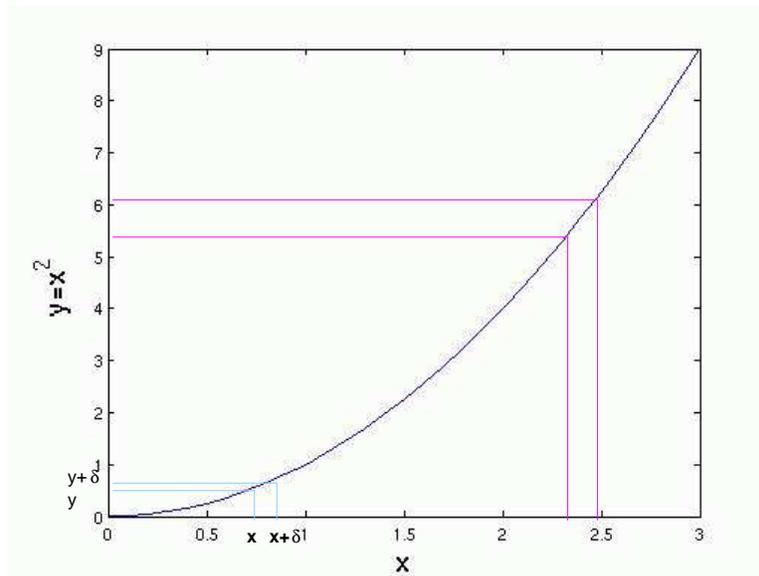
Figure 1: Example of uncertainty estimates for a parabola. Light blue straight vertical lines indicate position of  $x_o$  and  $x_o + \delta_{x_o}$ . Horizontal lines show corresponding difference in  $y(x_o)$  and  $y(x_o + \delta_{x_o})$ . Magenta lines show that if  $y$  has a steeper slope, then the difference between  $y(x_o)$  and  $y(x_o + \delta_{x_o})$  is greater, implying greater uncertainty.
