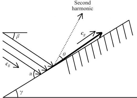
FIGURE 2. Schematic view of the reflection process for  $\gamma \approx \beta$ . The reflected wave is alongslope, whereas the nonlinearly reflected second harmonic, represented with the dotted line, makes an angle  $\theta$  with the slope.
