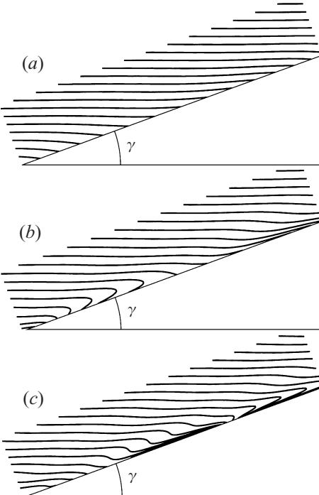
FIGURE 6. (a–c) Buoyancy field in the critical case at  $N \sin \beta t = 3, 10$  and  $20$ .  $\varepsilon = 0.3$ ;  $\beta = \gamma = 20^\circ$ . The dimensions of the panel are  $\lambda / \sin \alpha$  in the  $x$ -direction by  $\lambda / 5 \sin \alpha$  in the  $z$ -direction. In (b) and (c), some overturned regions are evident.
