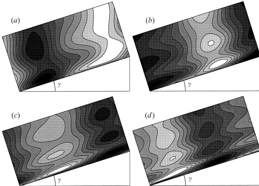
FIGURE 8. Streamfunction for four different times in the near-critical case:  $\beta = 22.58^\circ$ ;  $\gamma = 17.42^\circ$ ;  $\sigma = -1$ ;  $\varepsilon = 0.3$ . (a-d)  $N \sin \beta t = 5, 10, 15$  and  $20$ . The dimensions of the panel are  $\lambda / \sin \alpha$  in the  $x$ -direction by  $\lambda / 2 \sin \alpha$  in the  $z$ -direction.
