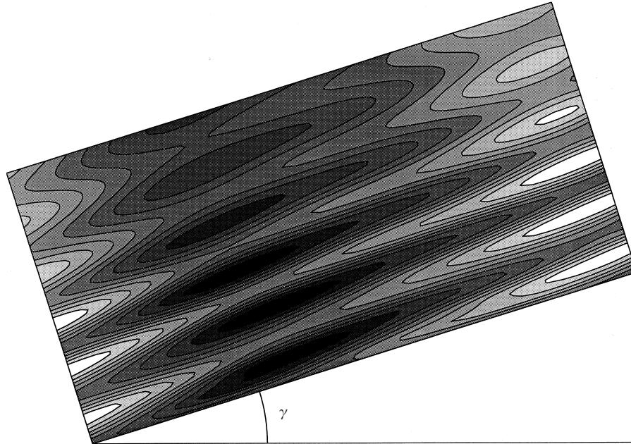
FIGURE 9. Streamfunction in the near-critical case at  $N \sin \beta t = 100$ ;  $\beta = 22.58^\circ$ ;  $\gamma = 17.42^\circ$ ;  $\sigma = -1$ ;  $\varepsilon = 0.3$ . The dimensions of the panel are  $\lambda / \sin \alpha$  in the  $x$ -direction by  $\lambda / 2 \sin \alpha$  in the  $z$ -direction.
