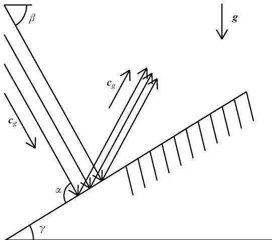
FIGURE 1. Schematic view of the reflection of the incident wave. The angle between the bottom slope and the horizontal is  $\gamma$ ; the angle between the incident group velocity and the horizontal is  $\beta$ , and  $\alpha = \beta + \gamma$ .  $c_g$  indicates the group velocity and  $g$  indicates gravity.
