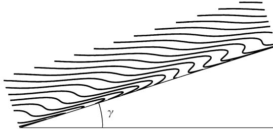
FIGURE 10. Buoyancy field at  $N \sin \beta t = 20$  in the near-critical case  $\beta = 22.58^\circ$ ;  $\gamma = 17.42^\circ$  and  $\varepsilon = 0.3$ . The dimensions of the panel are  $\lambda / \sin \alpha$  in the  $x$ -direction by  $\lambda / 5 \sin \alpha$  in the  $z$ -direction.
