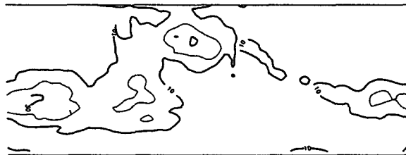
FIG. 18. Case M2: Time-mean eddy kinetic energies. Top: layer 1, and bottom: layer 2. CI = 10 \text{ m}^3 \text{ s}^{-2} .
