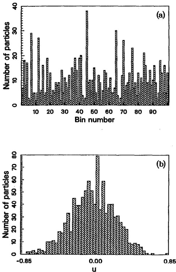
FIG. 8. (a) This figure shows a more detailed view of the particle density in Fig. 7(d). The position axis,  $0 < x < 1$ , is divided into 100 bins and the number of particles in each bin is counted. There is obvious clumping and, indeed, the largest agglomerations are unchanged if the bin size is halved. (b) The velocity distribution of the particles from Fig. 7(d).
