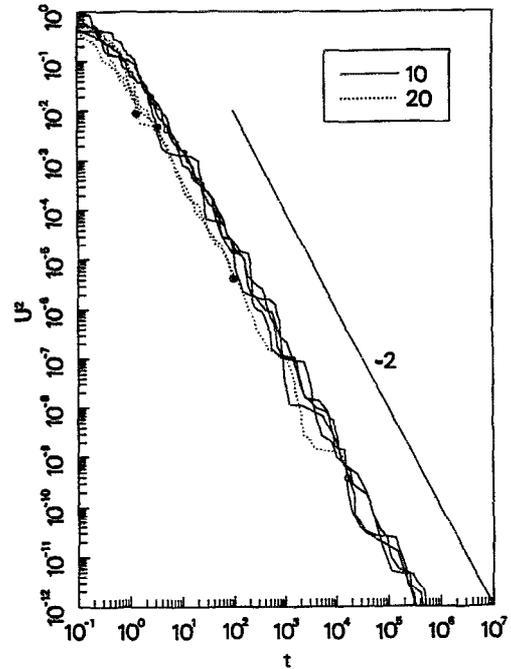
FIG. 4. The mean square velocity as a function of time for a cooling inelastic gas with  $r = 0.8$ . We show four realizations with  $N = 10$  and 20. The  $t^{-2}$  regime is clear for realizations with  $N = 10$ . But in the other cases, the  $t^{-2}$  regime is transient and is halted by inelastic collapse (indicated by the heavy dots).
