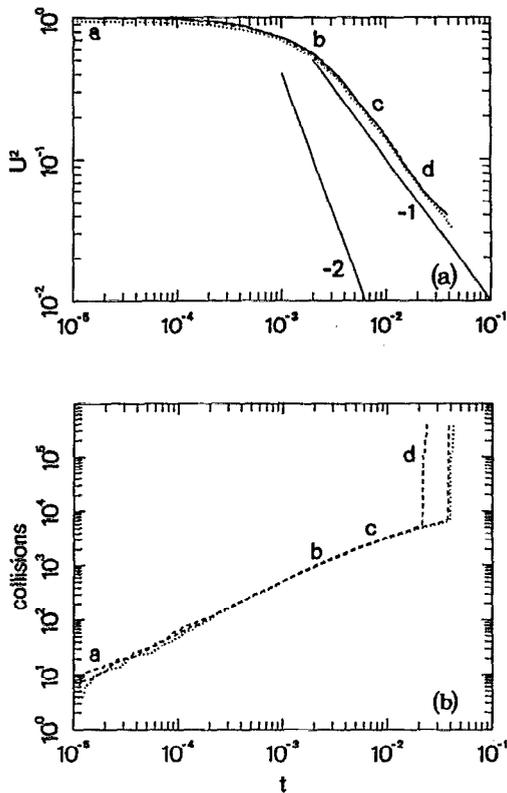
FIG. 6. Three realizations of a cooling simulation with  $r=0.8$  and  $N=1000$ . (a) The granular temperature as a function of time. There is a rough  $t^{-1}$  fit but, because collapse brings all of the simulations to a halt, this tentative regime is not convincingly demonstrated. (b) Collision number as a function of time. The vertical rise indicates that collapse has occurred.
