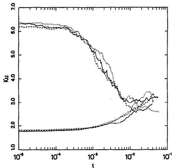
FIG. 9. The kurtosis, defined in Eq. (10), as a function of time for six realizations of the  $r = 0.8$  and  $N = 1000$  inelastic gas. The three simulations that begin with  $Ku \approx 1.8$  are the three simulations in Fig. 6. The other three have a piecewise constant initial velocity distribution, constructed to give  $Ku \approx 6$  and  $U^2 \approx 1$ . By collapse time, all six realizations are close to the Gaussian value  $Ku = 3$ .
