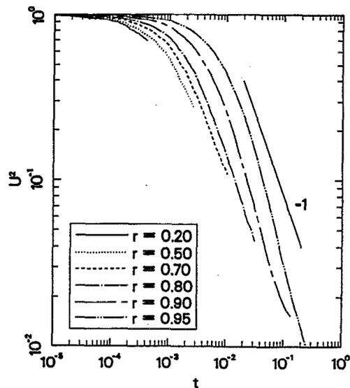
FIG. 10. Cooling laws for  $N = 1000$  particle gases with various coefficients of restitution  $r$ . In all six cases, the simulations are halted by inelastic collapse. There is some evidence of a transient scaling regime with a slope that steepens as  $r$  approaches 1.
