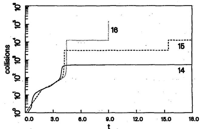
FIG. 3. Number of collisions as a function of time for three calculations. The curves labeled "14" and "15" refer to the simulations in parts (a) and (b) of Fig. 2. In both of these cases, the particles eventually disperse and the total number of collisions is finite. By contrast, the curve labeled "16" summarizes a calculation in which a cushion of 15 stationary particles is struck by a rapidly moving particle. In this case, inelastic collapse occurs at  $t \approx 9.0$ .
